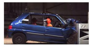
In the above photographs, L<sub>1</sub> is the original length of the car and L<sub>2</sub> is the length of the car after the crash. Thus, the crush distance  $d = L_1 - L_2$ .
